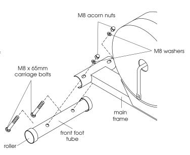
Figure 1 - Install Front Foot Tube
